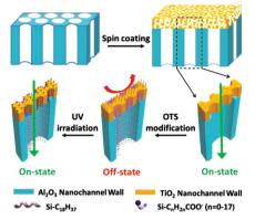
Artificial nanochannels based on chemically modified TiO2/Al2O3 heterogeneous porous membranes are described. The irreversible decomposition of octadecyltrimethoxysilane (OTS) molecules by TiO<sub>2</sub> photocatalysis under ultraviolet light results in a change of surface wettability and an asymmetric distribution of surface negative charges simultaneously, which contributes to the ion gating and regulatable ion rectification.
