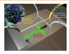
Using microfluidics to precisely regulate self-assembly conditions, a number of nanoparticle properties are tuned to optimize drug-delivery efficacy. These parameters include size, zeta potential, and pH responsiveness. These nanoparticles are stable during circulation at physiological pH, but if they encounter a tumor cell, where the pH is lower, they rapidly release their anti-cancer drug cargo.
