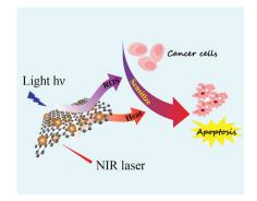
With the aid of sequential irradiation, highly integrated reduced graphene oxide-ZnO nanoparticle-hyaluronic acid nanoassemblies can serve as a multisynergistic platform for targeted highperformance apoptotic cancer therapy. The reactive oxygen species generated by ZnO/rGo under light irradiation can effectively sensitize cancer cells to the subsequent NIR laser-induced apoptotic hyperthermia.
