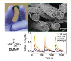
Flexible sensory material based on conformal multi-walled carbon nanotube (MWNT) films on a porous electrospunpolymeric fiber mat is constructed using a vacuum-assisted spray layer-by-layer assembly. The resulting thin MWNT films coat individual electrospun fibers with controlled loading and electrical conductivity. The MWNT/electrospun fiber electrodes display reversible responses and high sensitivity for detecting DMMP in aqueous and vapor phases.
